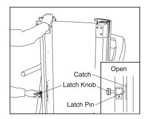
Hold the metal frame firmly with both hands, and lower the frame to the floor. CAUTION: To decrease the possibility of injury, do not lower the frame by gripping only the plastic foot rails. Do not drop the frame to the floor. Make sure to bend your legs and keep your back straight.
